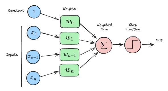
A logic gate is similar to a perceptron in that it also can be used as a binary linear classifier. With XOR, it takes on the implementation of a multi-layer perceptron, but the main concept within leveraging logic gates as perceptrons is that they both function as binary linear classifiers as demonstrated below:
